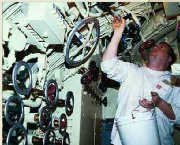
While the exterior finish required two shades of grey, 10 color shades were necessary inside in part because valve handles that had various functions were color-coded.
